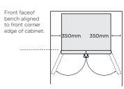
When positioned least 350mm on the hinge side will allow the doors to open enough to enable the removal of bins and shelves.
