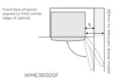
WTE & WTM models When positioned in a corner area, clearance (S) of at least 350mm on the hinge side will allow the doors to open enough to enable the removal of the crisper bins and shelves. This required clearance inceases to 550mm for those models with telescopic extension slide-out bins.
