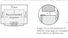
When positioned in a corner, the clearance must be at least 300mm on the hinge side to allow the door to open smoothly so that bins and shelves can be removed easily. For easy removal of Crisper it is recommended to remove bottle door bin first if minimum clearance in the corner on hinge side is less than 350mm.
