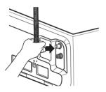
3 Adjust the band clamp with pliers to keep the hose securely in place and prevent leaking.
