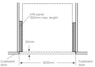
Infill panels are recessed 20mm from the external cabinet door to accommodate flush fit.
