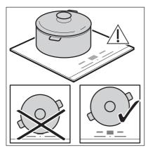
Place the cookware in the centre of the selected zone. Induction cooking zones adapt to the dimension of the bottom of the cookware automatically.
