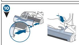
Replace the Brush Window by first lining up the Brush Window tabs with the edges of the foot. Then press the window back into place until you hear a click.
