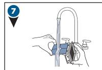
Hand wash the Vacuum Filter and Screen with warm water and mild detergent.
