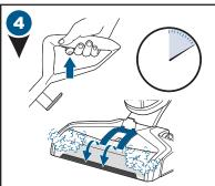
Before each use, hold the Solution Spray Trigger for 10 seconds to prime the system with cleaning solution. LED lights illuminate when holding the trigger.
