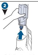
Lift the Clean Water Tank straight up to remove from the machine.
