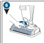
Grasp Brush Window at the front of the window and pull upward to remove.
