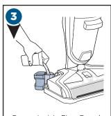
Pour water into Rinse Funnel to fill the MAX line of the Rinse and Storage Tray.
