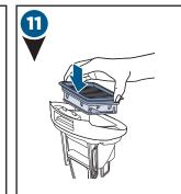
Place Vacuum Filter back into the top of the Dirty Water Tank.
