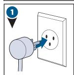
Plug machine into a properly grounded outlet.
