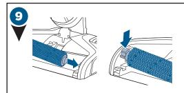
Replace Brush Roll by inserting the Brush Roll end into the right side of the foot. Then lock the pull tab into place by pressing downward.
