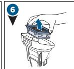
Remove the Vacuum Filter and Screen from the top of the Dirty Water Tank by pulling it up.
