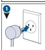
Plug machine into a properly grounded outlet.
