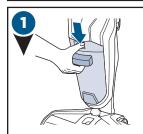
To release Dirty Water Tank, press down on recessed button on the top of the tank.
