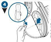
Then, with the mop pad folded, line up the small dot in the center of the pad with the middle screw on the bottom of the foot.
