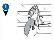
To remove mop pads, simply pull pads off the hook and loop material on the bottom of the machine.
