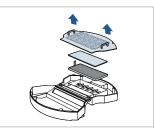
3. Remove the filter cover, then the foam and pleated filters.
