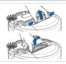
1. Turn the Power Switch OFF. Pinch the tabs on the brush guard inward and pull to remove. Lift to remove the Brush Roll
