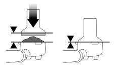
As a guide, the top edge of the cap on the tamper should be level with the top of the filter basket AFTER the coffee has been tamped.
