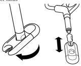
Rinse the steam tip and wipe with a clean, dry cloth. Reassemble the steam wand by screwing the steam tip back on to the steam wand. Purge the steam wand after cleaning.
