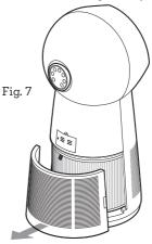
2. Remove the used filter using the pull tabs on the filter (Fig 8).
