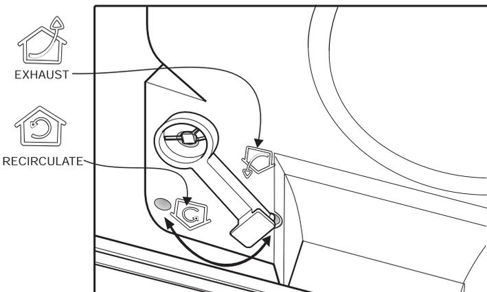
**IMPORTANT: SET CIRCULATING MODES BEFORE INSTALLING THE HOLE PLUGS.**
