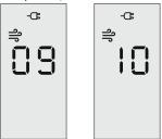
Press the speed button ▲ or ▼ (L) to increase or decrease the fan speed (within 4/5 seconds) the display will show the fan speed.
