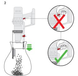
Be careful not to pull the 'ON' trigger while the clear bin is open for emptying.
