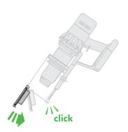
Close the clear bin by pushing the bin base upwards until the clear bin and bin base click into place.
