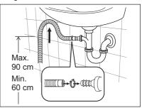
Push the drain hose onto the spigot and secure with a clamp, ensure a loop is formed in the drain hose to prevent waste from the sink entering the appliance.
