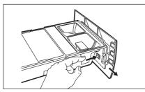
Make sure that all detergent residue is removed from the upper and lower part of the recess. Use a small brush to clean the recess.
