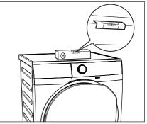
If you do not have a spirit level, as a guide use the edge of a door frame, cupboard or bench to check that the washing machine is leveled. Loosen or tighten the feet to adjust the level. A correct adjustment of the appliance level prevents vibration, noise and the movement of the appliance when in operation.
