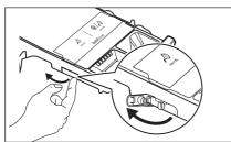
4. Press the catch on the back as indicated in the picture and lift up the top cover to remove it.
