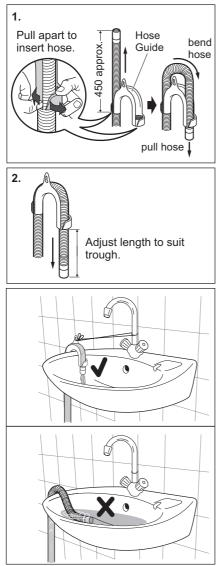
In this case, make sure the end cannot come unhooked when the machine will be emptied. This could be done by tying it to the tap with a piece of string or attaching it to the wall.
