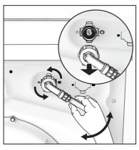
5. Use a suitable tool pulling filter from the valve (eg. long nose pliers) as picture.
