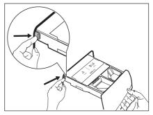
2. Remove the insert for the softener and, if inserted, the special container for liquid detergent.
