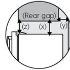
If you have a cupboard above the refrigerator with a rear gap of less than 100 mm (Y), recommended clearance at the top of the refrigerator increases from 50mm to 90mm (X) minimum.
