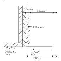
**NOTE:** Your appliance must be mounted on a flat horizontal surface for the full width and depth of the product
