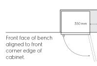
When positioned in a corner area, spacing of at least 400mm on the hinge side will allow the doors to open enough to enable the removal of bins and shelves.
