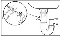
Fix the water drain hose properly to the piping. The hose has to reach at one point a height between 400 and 850 mm above the appliance bottom line!
