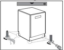
I. Install the appliance on solid ground. Adjust accurately all feet to get a firm, horizontal position.
