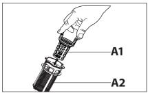
A B I. Turn the filter **A** anticlockwise and remove it.
