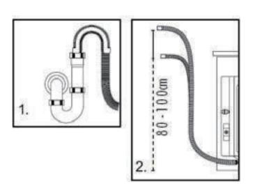
A The drain hose should not be submerged in water and should be securely fixed and leak-free. If the drain hose is placed on the ground or if the pipe is at a height of less than 80cm, the washing machine will con tinuously drain while being filled (self-siphoning).
