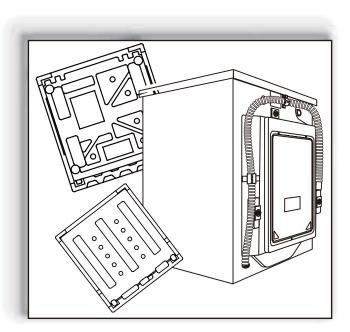
Remove all the packing materials to prevent unsteadiness, including the polystyrene base. Upon opening the package, water drops may be seen on the plastic bag and the porthole. This is normal phenomenon resulting from water tests in the factory.
