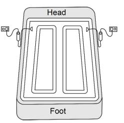
**WARNING:** Failure to follow these fitting instructions may trigger the overheat system and render the blanket permanently inoperative. This may invalidate the warranty.
