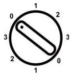
To turn on the fan, turn the speed control switch (1) to positions 1, 2 or 3 according to the desired speed you need. By turning the switch to the positions 1,2,3 you can adjust the wind speed of the fan. To turn off the fan, just turn the switch to position "0".
