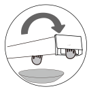
1. Take out the water box horizontally to avoid spllover of condensate water.
