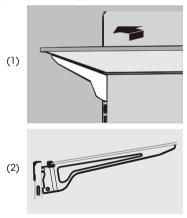
To reinstall a shelf, gently slide the shelf back into the refrigerator compartment, and lower the shelf onto the rail support.
