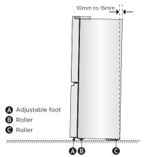
NOTE: Having someone push against the top of the refrigerator takes some weight off the leveling feet. This makes it easier to turn the feet. Rotate the adjustable feet clockwise to raise or counter-clockwise to lower your refrigerator. To make sure that the doors close automatically, till the top of your refrigerator backward about 10mm to 15mm. If necessary, use a spanner wrench to adjust the feet.
