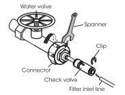
To prevent the clips loose, use the valve seat to hold it. Then use the screw to hold the valve seat with Philips(+) screwdriver.
