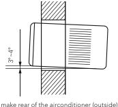
lower than the front of the airconditioner (outside) lower than the front of the airconditioner (inside) to allow water to drain
