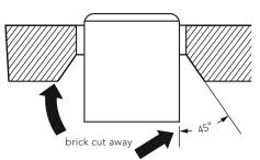
if the wall thickness is more than 220mm 45° brick cut away to install louvres properly.
