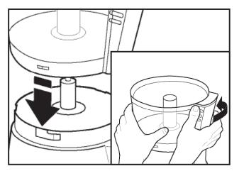
**3.** Fit the blade over the shaft in the center of the work bowl, rotate, and press down until it locks into operating position.
