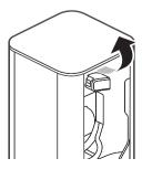
2 To insert, align the battery with the outline of the battery charger.
