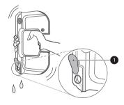
2 Leave the water inlet cap open and allow the water tank to dry in a well-ventilated area out of direct sunlight for at least 24 hours.
