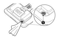
1 Open the 2 water inlet caps ① on the side of the water tank and empty the water tank. Shake the water tank to remove the remaining water. Do not tap the water tank against any surface.
