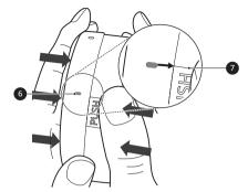
8 Push and insert the exhaust filter cover **3** into the exhaust filter **1** and rotate it to reassemble it and prevent it from falling out.
