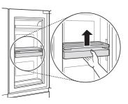
2 To lower the moving basket, press up to release the levers at the side of the basket and lower the basket until it clicks into place.
