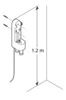
**3** Attach the charging station to the wall with the wall anchoring screws.
