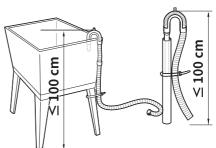
• If the drain hose is too long, do not force it back into the appliance. This will cause abnormal noise.
