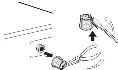
**Cleaning the Drain Pump Filter and Performing an Emergency Water Evacuation**
