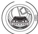
**4** Place wet items on top of the rack. Allow space around items for air to circulate.
