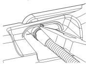
4 Loosen the screw 2 on the stack bracket.
