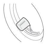
Reinsert both inner and outer filter and close the dryer's door.
