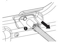
3 Connect the drain hose of the dryer and secure the hose clamp.
