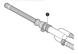
4 Connect securely the short drain hose to a floor gully or a standpipe.
