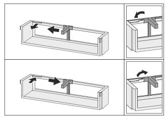
Disassemble the door rack.
