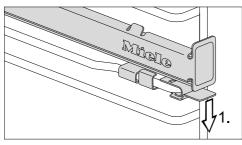
Push down on the tab at the front of the FlexiClip telescopic runner (1.).
