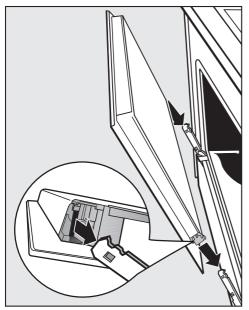
Hold the door securely on both sides and carefully fit it back onto the hinge retainers.
