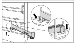
Hook the FlexiClip telescopic runner onto the front of the top rail of a shelf runner (1.).
