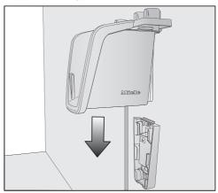
Slide the wall bracket down into the mounting plate from above until it audibly clicks into place.
