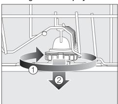
■ Rotate the screw thread of the middle spray arm clockwise (overhead perspective) ① (see diagram) and remove the spray arm ②.
