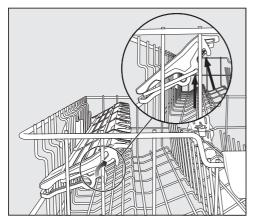
■ Pull the cup rack upwards and click it into the desired position (see arrows).
