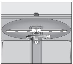
■ Push the upper spray arm upwards ① to engage the inner ratchet. Then unscrew the spray arm by rotating the screw thread anti-clockwise (when viewed from below) ②.
