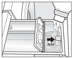
■ Add fabric softener or liquid starch to the ℜ compartment. **Do not exceed the maximum level mark.**
