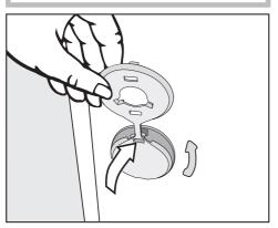
■ Fit the stoppers onto the two holes.
