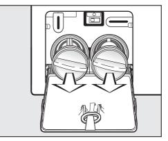
Remove the filters completely.
