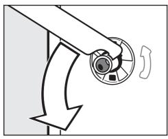
Using the spanner supplied, turn the left-hand transit bar anti-clockwise 90°, then
