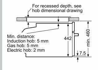
measurements in mm
