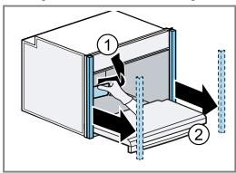
2. Turn the fastening element to the left or right to adjust the alignment of the panels.
