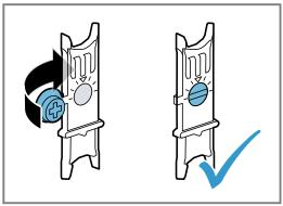
2. Hook in the fastening element at the bottom and press down at the top until it is in place.
