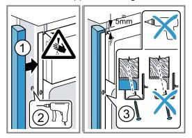
**Note:** The gap between the worktop and the appliance must not be sealed by additional strips.
