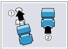
Hook the rear retainers with the hook into the top hole ① and push them into the bottom hole ②.
