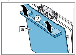
6. Set the front pane down on a level surface with the door handle facing down.
