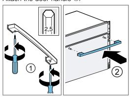
4. Tighten the screws until the door handle is secured.
