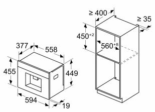
Bean and water containers are removed from the front Recommended installation height
