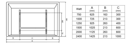
**WARNING -** Minimum clearances and IP zone requirements must be adhered to. Do not locate the heater immediately below a fixed electrical power point.
