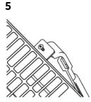
To secure the heater safely to the wall, fasten the screw on each of the two catches at the top of the wall bracket.
