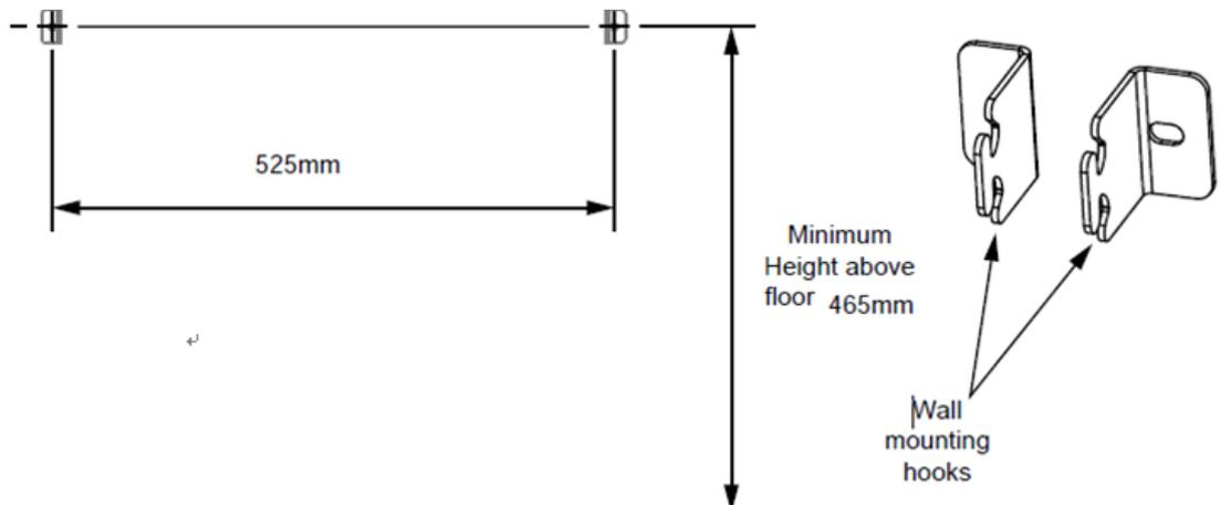
Attach the supplied right angle mounting brackets to the underside of the heater (front hole of bracket) using the rear most of the pre installed case screws as shows in the diagram. Check for strength.
