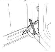
2. Grasp the door on both sides with both hands, lift it forming an angle of around 30° and remove it.
