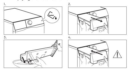
You can use the water from the water container as an alternative to distilled water (e.g. for steam ironing). Before you use the water, remove dirt residues with a filter.
