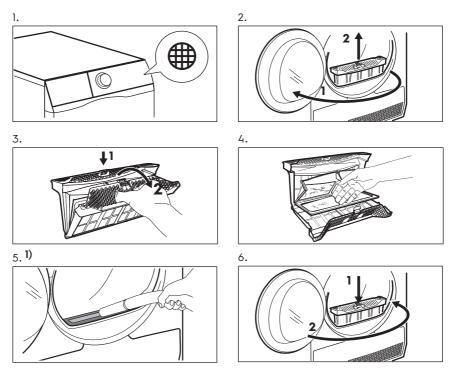
1) If necessary remove fluff from the filter socket and gasket. You can use a vacuum cleaner.
