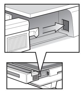
• Push the middle of the trim down to ensure it is straight and firm against the glass panel.
