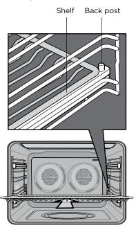
2. Drop the front of the shelf or tray onto the slide ensuring it sits behind the front post of the slide.
