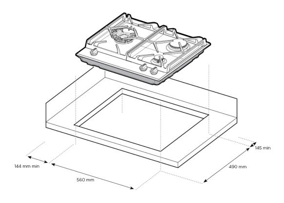
NOTE: Distances shown to adjacent walls/surfaces are for the distance to a combustible surface. If the surface is not combustible the measurement can be smaller than that shown.
