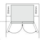
When positioned In a corner area, spacing of at least 350mm on the hinge side will allow the doors to open enough to enable the removal of bins and shelves.
