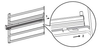
3. Push slide front clip over wire until secured
