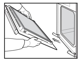
Lay the oven door with the outer side facing downwards on something soft and flat (for example a blanket on a kitchen table) to prevent scratches.
