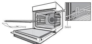
4. When fully inserted the shelf should not interfere with the closed oven door.
