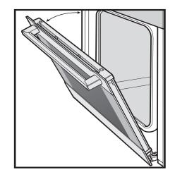
Grasp the oven door with a hand each side of the door and remove it from the oven by pulling it towards you.
