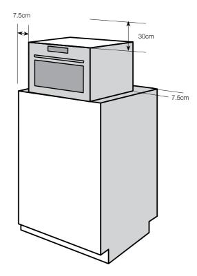
Blocking the intake or outlet vents can damage the oven. If air vents are blocked during operation, the oven may overheat, and this may lead to malfunctioning. Hot air escapes from the vents, so be sure not to obstruct it or let curtains come between the oven and the rear wall.
