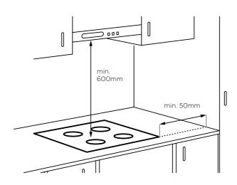
NOTE: The clearance must meet or exceed the minimum recommended for both the rangehood and cooktop. Refer to the rangehood installation manual.
