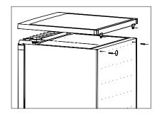
2. Remove the four screws as follow diagram. Lift the upper hinge core, then put it in a safe place.
