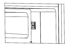
4. Turn the freezer compartment door through 180°, cover the cap on the up door bearing, then fit the door into the up door axle hole.
