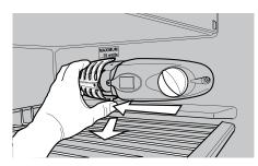
Unscrew the spent light bulb in an anti-clockwise direction.
