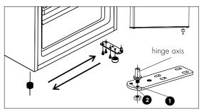
4. Set the door into its new place making sure the pin enters the bushing at the lower frame section. Replace the lid by fitting the upper hinge core into the upper door's hole, securing it with the two screws. Replace another two screws to another side.
