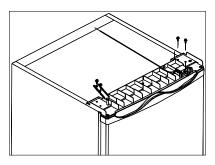
5. Put the top cover in the freezer. Tighten the two screws on the back of top cover.
