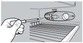
3. Remove the light lens by pushing back and down on the clear plastic tab protruding from the bottom of the lens.
