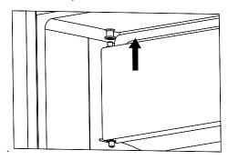
Keep the freezer compartment door closed. Fix the installation button to the lower door bearing, Press the installation button to make it have no gap with the cavity, then fix the screw.
