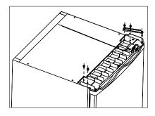
3. Lift the door and place it on a padded surface to prevent scratching. Remove both adjustable feet and remove the bottom hinge bracket by unscrewing the bolts. Then transfer them to another side.
